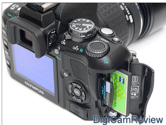
Back - 2.5" screen, Optical viewfinder with diopter correction, Playback mode, delete, menu, info, AEL/AFL, Function button (can be customised, but in custom white balance mode, holding it and taking a photo will set the custom white balance for you), 4-way controller, OK button in middle. Dual Compact flash / XD Memory card compartment. USB socket cover.
