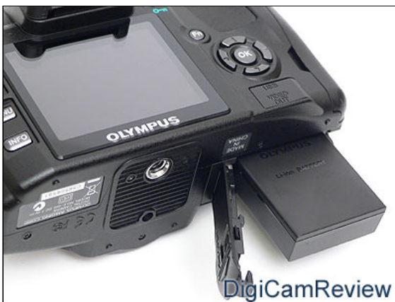
Left / Top: Flash hotshoe, Mode dial. On/Off, exposure compensation button, shutter, control dial (corner), pop-up flash and button, shooting mode. Right / Bottom - battery compartment (open/close latch), metal tripod mount.
