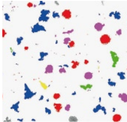
Fig. 3: One typical analytical metallography task is investigating graphite in cast iron. Using image-analysis methods for evaluation, each graphite particle is automatically detected and its shape and size evaluated. The size and shape distribution of all particles is displayed in tables and diagrams. Classifications according to national and international standards such as VDG, EN ISO, JIS or ASTM are integrated. In addition, the carbon-corrected ferrite/pearlite ratio can be determined.
